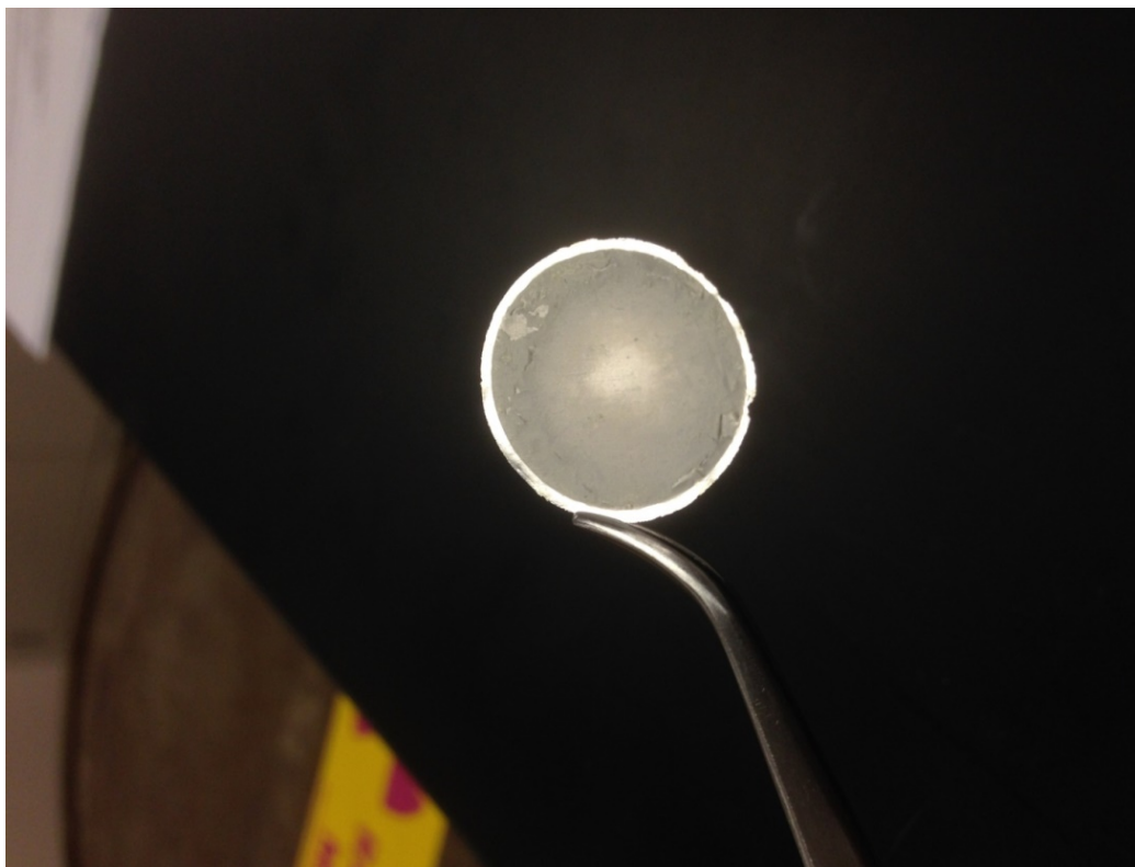
Fig. 1. Picture of Al-disk after stable Nb electrodeposition.
